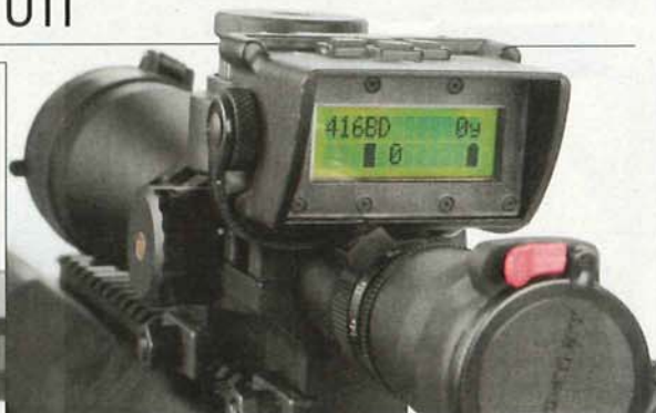
The simple LCD screen displays the particular load, battery condition, the range, and whether or not the rifle is level.
